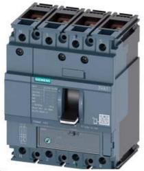
CIRCUIT BREAKER 3VA1 IEC FRAME 160 BREAKING CAPACITY CLASS N ICU=25KA @ 415 V 4-POLE, LINE PROTECTION TM220, ATFM, IN=100A OVERLOAD PROTECTION IR=70A ...100A SHORT CIRCUIT PROTECTION II=10 X IN NEUTRAL UNPROTECTED BUSBAR CONNECTION
