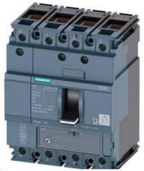
CIRCUIT BREAKER 3VA1 IEC FRAME 160 BREAKING CAPACITY CLASS H ICU=70KA @ 415 V 4-POLE, LINE PROTECTION TM220, ATFM, IN=63A OVERLOAD PROTECTION IR=44,1A ...63A SHORT CIRCUIT PROTECTION II=10 X IN NEUTRAL UNPROTECTED CABLE CONNECTION
