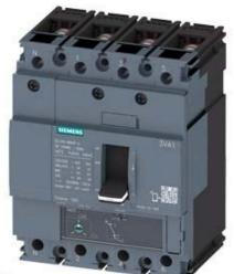
CIRCUIT BREAKER 3VA1 IEC FRAME 160 BREAKING CAPACITY CLASS H ICU=70KA @ 415 V 4-POLE, LINE PROTECTION TM220, ATFM, IN=63A OVERLOAD PROTECTION IR=44,1A ...63A SHORT CIRCUIT PROTECTION II=10 X IN NEUTRAL PROTECTION 100% BUSBAR CONNECTION
