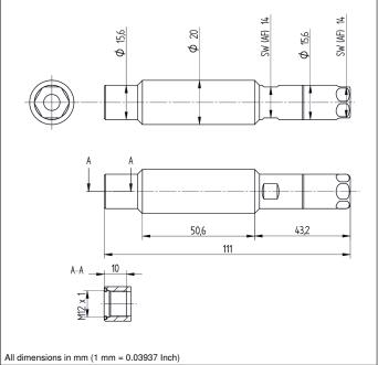
InoxSens is the hygiene series from wenglor. The InoxSens mounting tubes are also part of this complete system, which is seamlessly integrated into the machine. The stainless steel tubes made of V4A (1.4404/316L) are corrosion-free and resistant to cleaning agents, and they provide IP68/IP69K protection for all standard connector cables.
