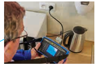
3-pole cable for direct measurements on 2P+E sockets.
