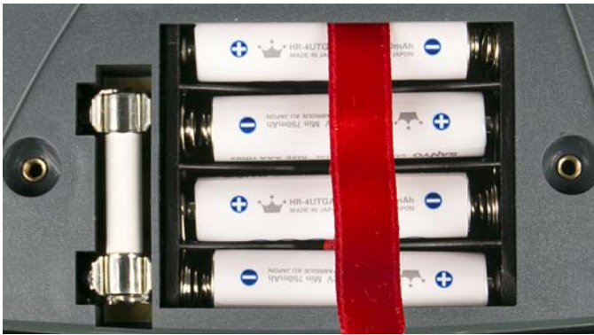
Figure 5: Correct Battery Polarity
