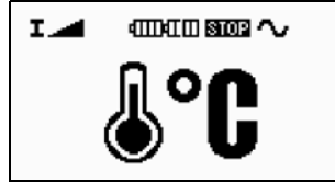
Figure 3.11: Indication of Overheating After Pressing the START Key
