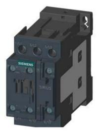
CONTACTOR, AC-3, 15KW/400V, 1NO+1NC, DC 24V, 3-POLE, SZ S0 SCREW TERMINAL UPRIGHT MOUNTING POSITION
