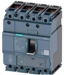
CIRCUIT BREAKER 3VA1 IEC FRAME 160 BREAKING CAPACITY CLASS M ICU=55KA @ 415 V 4-POLE, LINE PROTECTION TM240, ATAM, IN=20A OVERLOAD PROTECTION IR=14A ...20A SHORT CIRCUIT PROTECTION II=5 X IN NEUTRAL PROTECTION 100% BUSBAR CONNECTION
