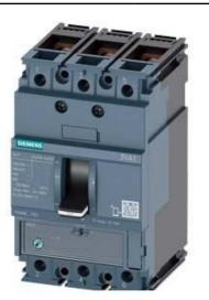
CIRCUIT BREAKER 3VA1 IEC FRAME 160 BREAKING CAPACITY CLASS H ICU=70KA @ 415 V 3-POLE, LINE PROTECTION TM220, ATFM, IN=40A OVERLOAD PROTECTION IR=28A ...40A SHORT CIRCUIT PROTECTION II=10 X IN BUSBAR CONNECTION
