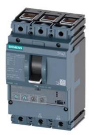
CIRCUIT BREAKER 3VA2 IEC FRAME 100 BREAKING CAPACITY CLASS M ICU=55KA @ 415 V 3POLE, LINE PROTECTION ETU350, LSI, IN=25A OVERLOAD PROTECTION IR=10A ...25A SHORT CIRCUIT PROTECTION ISD=1,5... 10 X IR, II=12 X IN CABLE CONNECTION
