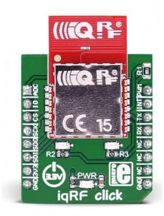
**IQRF click** carries the <u>DCTR-76DA</u> RF transceiver, operating in the 868/916 MHz frequency.
