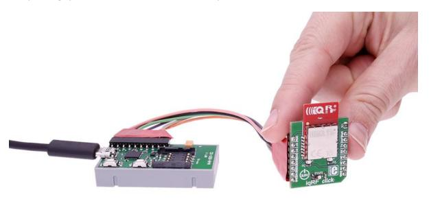
To upload application codes in DCTRs and configure DCTR parameters, <u>CK-USB-04A kit</u> is intended. When the application is uploaded to the IQRF it can be put in microBUS™ socket and communicate with it with MCU.
