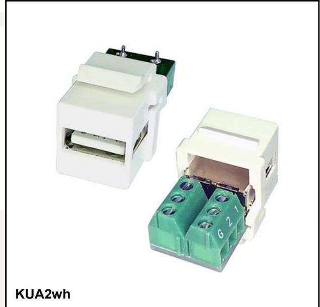
Suitable for field termination, repair and prototyping applications this 'DIY' socket enables an easy termination where a USB port is required. The 'breakout' board brings out all signal pins and the shield to screw-down terminal blocks for simple and reliable connection without the need for special tools.
