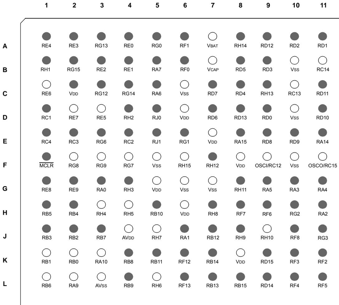
**Legend:** Shaded balls indicate pins tolerant to up to +5.5 VDC. See [Table 5](#) for a complete description of pin functions.
