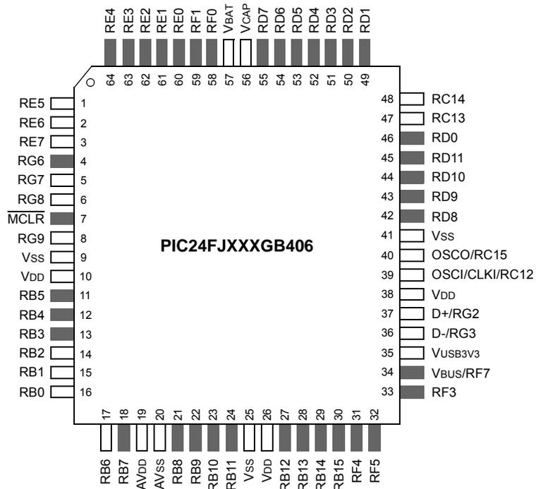
**Legend:** Shaded pins indicate pins tolerant to up to +5.5 VDC. See [Table 2](#) for a complete description of pin functions.
