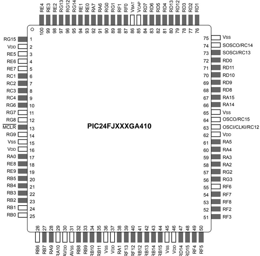
**Legend:** Shaded pins indicate pins tolerant to up to +5.5 VDC. See [Table 3](#) for a complete description of pin functions.
