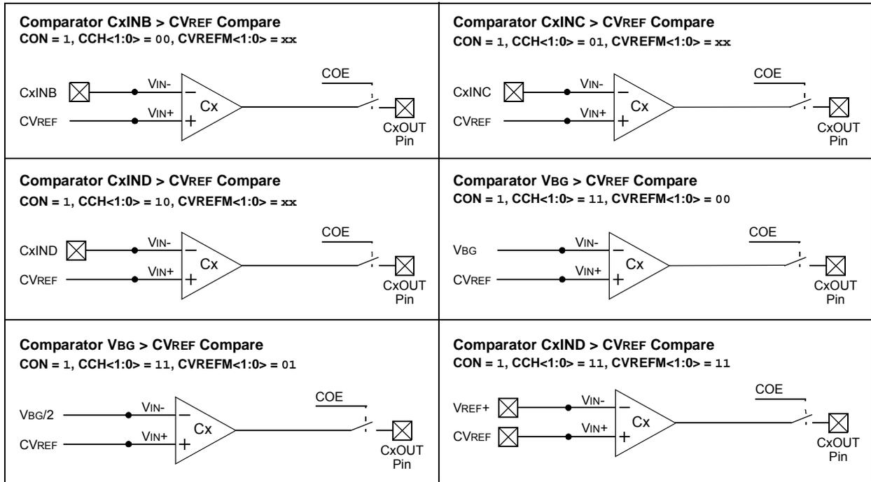
**FIGURE 29-4: INDIVIDUAL COMPARATOR CONFIGURATIONS WHEN CREF = 1 AND CVREFP = 1**
