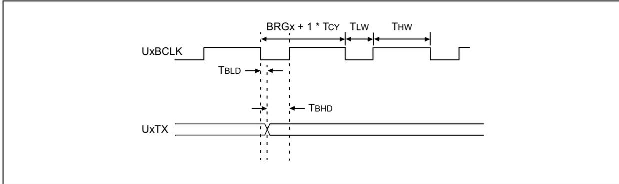
**FIGURE 36-18: UARTx START BIT EDGE DETECTION**
