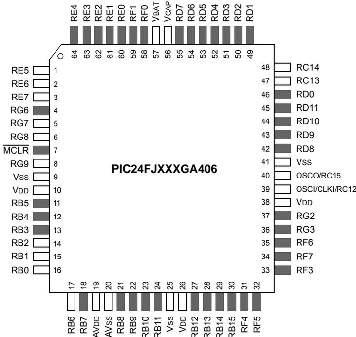
**Legend:** Shaded pins indicate pins tolerant to up to +5.5 VDC. See [Table 1](#) for a complete description of pin functions.
