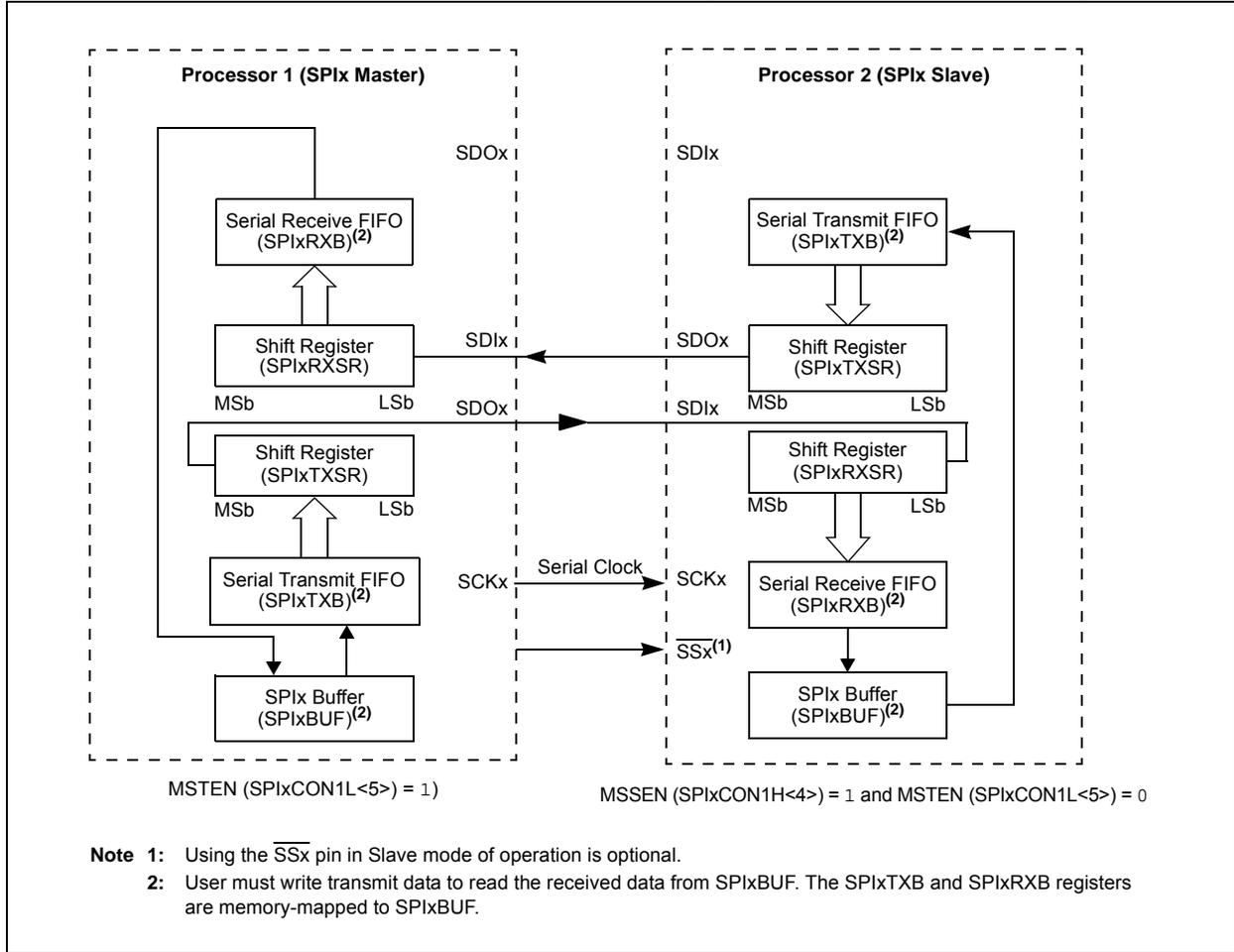
**FIGURE 17-5: SPIx MASTER, FRAME MASTER CONNECTION DIAGRAM**
