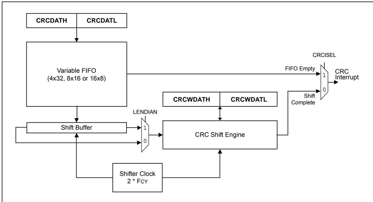
FIGURE 26-2: CRC SHIFT ENGINE DETAIL
