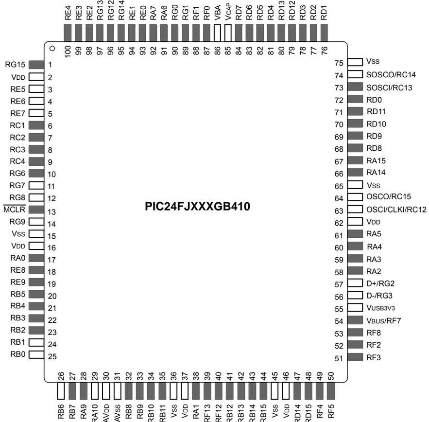
**Legend:** Shaded pins indicate pins tolerant to up to +5.5 VDC. See [Table 4](#) for a complete description of pin functions.
