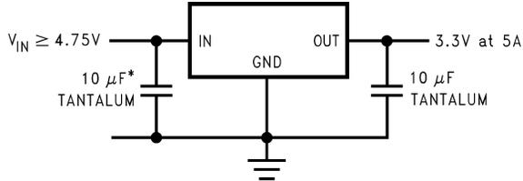
\*MAY BE OMITTED IF INPUT SUPPLY IS WELL BYPASSED WITHIN 2" OF THE LM1084
