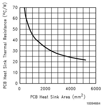
FIGURE 7. Heat sink thermal Resistance vs Area
