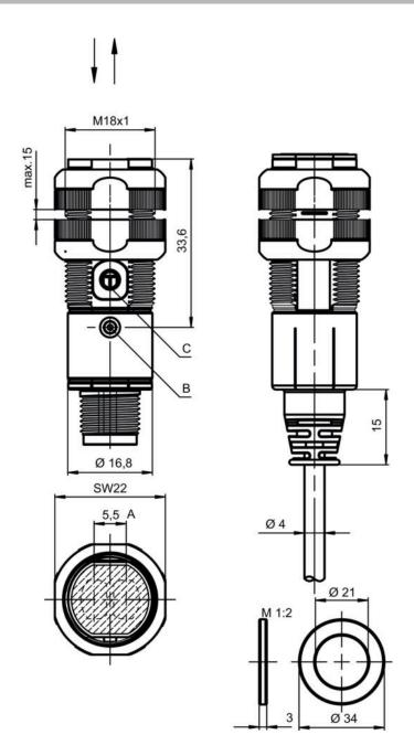
A Optical axis B Indicator diode
