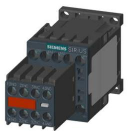
CONTACTOR, AC-3, 3KW/400V, 2NO+2NC, DC 24V, 3-POLE, SZ S00 SCREW TERMINAL PERMANENT AUX. SWITCH FOR SUVA APPLICATIONS
