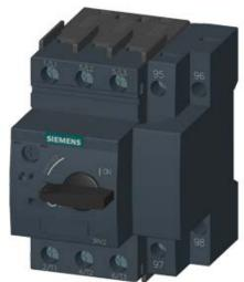
CIRCUIT-BREAKER SZ S00, FOR MOTOR PROTECTION, CLASS 10, W. OVERLOAD RELAY FUNCTION A-RELEASE 10...16A, N-RELEASE208A, SCREW CONNECTION, STANDARD SW. CAPACITY
