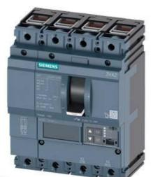
CIRCUIT BREAKER 3VA2 IEC FRAME 100 BREAKING CAPACITY CLASS L ICU=150KA @ 415 V 4POLE, LINE PROTECTION ETU550, LSI, IN=25A OVERLOAD PROTECTION IR=10A ...25A SHORT CIRCUIT PROTECTION ISD=0,6..10X IN, II=1,5..12X IN NEUTRAL PROTECTION ADJUSTABLE (OFF, UPTO 160%) CABLE CONNECTION
