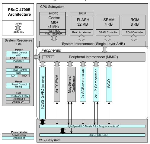
Figure 2. Block Diagram
