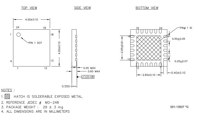
The center pad on the QFN package should be connected to ground (VSS) for best mechanical, thermal, and electrical performance. If not connected to ground, it should be electrically floating and not connected to any other signal.
