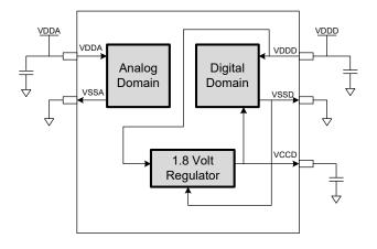
There are two distinct modes of operation. In Mode 1, the supply voltage range is 1.8 V to 5.5 V (unregulated externally; internal regulator operational). In Mode 2, the supply range is 1.8 V  $\pm$ 5% (externally regulated; 1.71 to 1.89, internal regulator bypassed).
