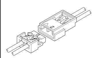
This is the wire-to-wire connector for DC power supply.
