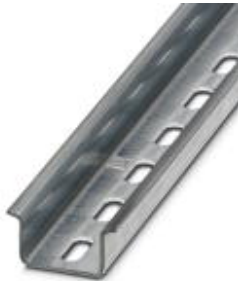
DIN rail, material: Galvanized, perforated, height 15 mm, width 35 mm, length: 2 m
