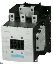
CONTACTOR, 75KW/400V/AC-3, AC(40...60HZ)/DC OPERATION UC 110...127V AUXIL. CONTACTS 2NO+2NC LATERAL, PERMANENT. JOINTED 3-POLE, SIZE S6 BAR CONNECTIONS CONVENTIONAL OPERATING MECHAN. FOR SUVA APPLICATIONS
