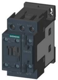
CONTACTOR, AC-3, 4KW/400V, 1NO+1NC, AC 230V 50HZ, 3-POLE, SZ SO SCREW TERMINAL
