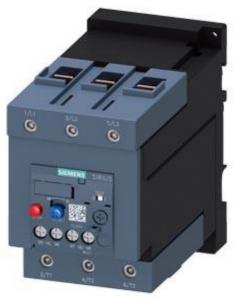
THERM. OVERLOAD RELAY 70...90 A FOR MOTOR PROTECTION SIZE S3, CLASS 10 FOR STAND-ALONE MOUNTING MAIN CIRCUIT: SCREW TERMINAL AUX. CIRCUIT: SCREW TERM. MANUAL-AUTOMATIC-RESET
