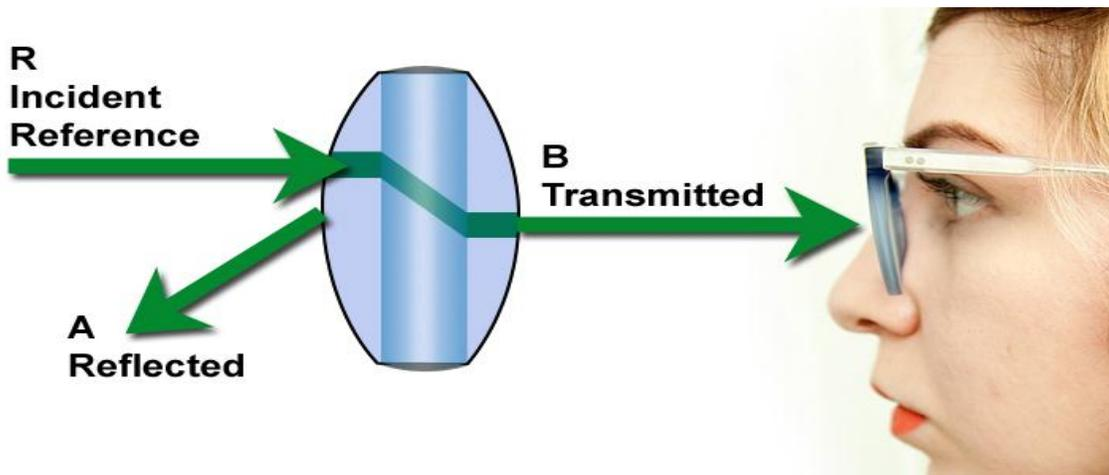
Here is a visual for S-Parameter data in an electrical circuit:
