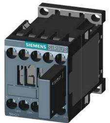
COUPLING CONTACTOR RELAY, 3NO+1NC, DC 24V, 0.85..1.85\*US, W/ PLUGGED-ON VARISTOR, SIZE S00, SCREW TERMINAL
