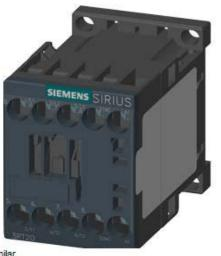
CONTACTOR, AC-3, 3KW/400V, 1NC, AC 380V 50/60HZ, 3-POLE, SZ S00 SCREW TERMINAL
