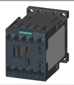
COUPLING RELAY, AC-3, 3KW/400V, 1NO, DC 24V, 0,85...1,85\*US, W. INTEGR. SUPPRESSORDIODE, 3-POLE SZ S00, SCREW TERMINAL
