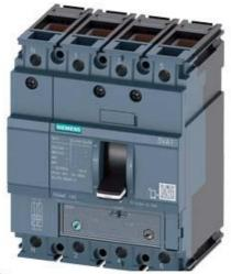
CIRCUIT BREAKER 3VA1 IEC FRAME 160 BREAKING CAPACITY CLASS M ICU=55KA @ 415 V 4-POLE, LINE PROTECTION TM240, ATAM, IN=160A OVERLOAD PROTECTION IR=112A ...160A SHORT CIRCUIT PROTECTION II=5...10 X IN NEUTRAL PROTECTION 50% CABLE CONNECTION
