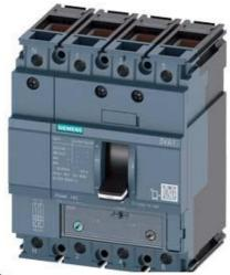
CIRCUIT BREAKER 3VA1 IEC FRAME 160 BREAKING CAPACITY CLASS N ICU=25KA @ 415 V 4-POLE, LINE PROTECTION TM240, ATAM, IN=20A OVERLOAD PROTECTION IR=14A ...20A SHORT CIRCUIT PROTECTION II=5...10 X IN NEUTRAL PROTECTION 100% CABLE CONNECTION
