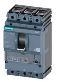
CIRCUIT BREAKER 3VA2 IEC FRAME 160 BREAKING CAPACITY CLASS M ICU=55KA @ 415 V 3POLE, LINE PROTECTION ETU350, LSI, IN=160A OVERLOAD PROTECTION IR=64A ...160A SHORT CIRCUIT PROTECTION ISD=1,5... 10 X IR, II=10 X IN CABLE CONNECTION
