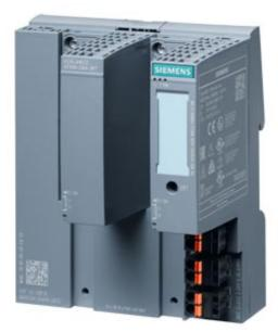
XF204-2BA IRT managed IE IRT Switch, 4 x 10/100MBit/s, 2 x bus adapter interface fault signal contact, with set button, redundant 24 V DC power supply, PROFINET IO Device, Network management, redundancy manager integrated, incl. electron. manual on CD-ROM, C-plug optional
