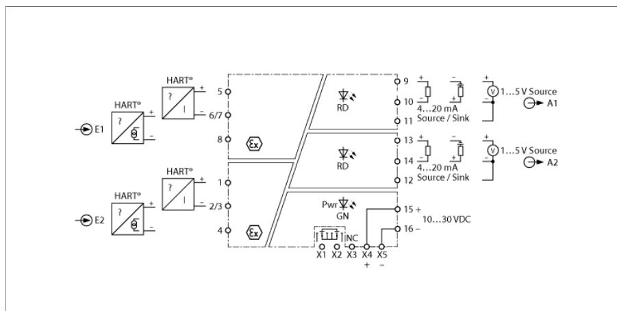
The 2-channel IMX12-AI01-2I-2IU-HPR/24VDC HART® isolating transducer is designed to operate intrinsically safe HART® 2-wire transducers in the Ex area and to transmit the measured signals to the non-Ex area. In addition to the analog signal also digital HART® communication signals can be transmitted bidirectionally. Alternatively, active 2-wire HART® transmitters and passive 3-wire HART® transmitters can be operated. The device can be powered from a power rail that also transmits a common alarm.
