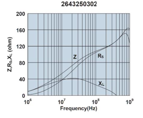
Impedance, reactance, and resistance vs. frequency.
