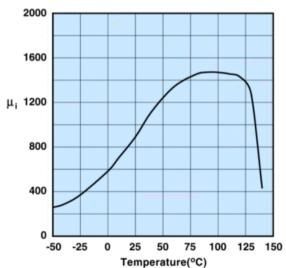
Measured on a 17/10/6mm toroid at 100kHz.
