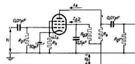
$R_a = 0,22$  M $\Omega$ ;  $R_{g1} = 1$  M $\Omega$ ;  $R_{g1}' = 0,68$  M $\Omega$ .
