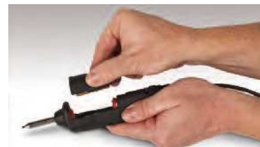
Collection chamber replacement
