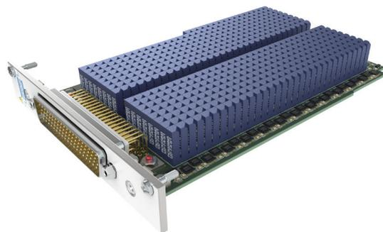
A total of 528 Series 120 relays on Pickering Interfaces ultra-high-density PXI module illustrates the packing density of these extremely small Reed Relays.
