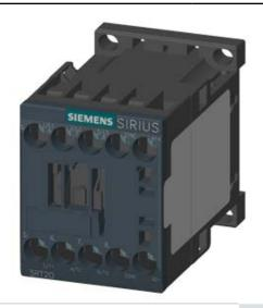
COUPLING RELAY, AC-3, 4KW/400V, 1NC, DC 24V, 0.7...1.25\*US, W. INTEGR. SUPPRESSORDIODE, SZ S00, SCREW TERMINAL
