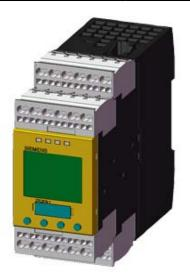
SIRIUS SAFETY RELAY SAFETY-RELATED SPEED MONITORING, 24 V DC, 45.0 MM, SPRING-LOADED TERMINAL, RC INSTANTANEOUS: 2NO RC DELAYED: 0 SC: 2 ELECTRICAL, AUTOSTART / MANUAL START, BASIC UNIT, MAX. ACH. PL EN13849-1: E, MAX. ACH. SIL TO IEC61508:3
