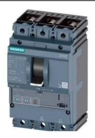
CIRCUIT BREAKER 3VA2 IEC FRAME 100 BREAKING CAPACITY CLASS L ICU=150KA @ 415 V 3POLE, LINE PROTECTION ETU320, LI, IN=40A OVERLOAD PROTECTION IR=16A ...40A SHORT CIRCUIT PROTECTION II=12 X IN BUSBAR CONNECTION
