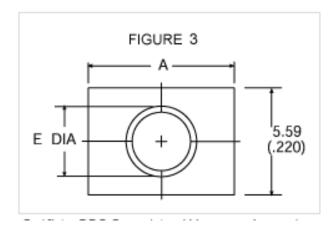
Polyphenylene Sulfide PPS Shoulder Washer. A single gate extension not to exceed 0.64mm (0.025) in length is allowable on the outside of all shoulder washers.
