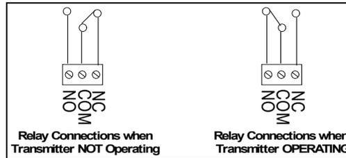
**The action of the relay outputs us set by Option link setting Jumper. A link is made / removed by the small shorting link 'cap' placed over the pin header.**
