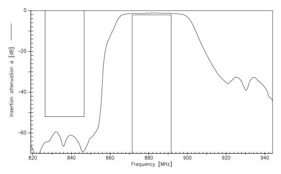
Transfer function for WCDMA signals (Power transfer function vs. carrier frequency)
