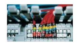
Helagrip cable markers have a specially designed profile, allowing each size to fit a wide range of cable diameters. The chevron end cut enables locked alignment of a series of legends. Helagrip is manufactured from a high-grade PVC compound and is indelibly marked.
