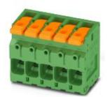
PCB terminal block, nominal current: 76 A, rated voltage (III/2): 1000 V, nominal cross section: 16 mm², Number of potentials: 2, Number of rows: 1, Number of positions per row: 2, product range: LPT 16/, pitch: 10 mm, connection method: Lever Push-in connection, mounting: Wave soldering, conductor/PCB connection direction: 0 °, color: green, Pin layout: Zigzag pinning W, Solder pin [P]: 3.6 mm, type of packaging: packed in cardboard
