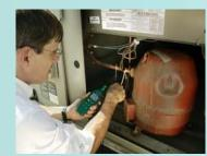
Compact meter is well-suited for field applications. Unique sensor cap closes for protection during storage. Simultaneously displays relative humidity, air temperature and dew point or wet bulb. Calculates T1-T2 differential (air temperature minus external probe temperature) using optional probe (TP890), and T2 minus dew point. Other features include Data Hold, Auto Power Off, and MAX/MIN reading.
