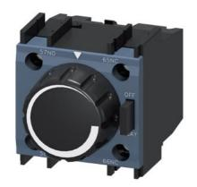
pneumatically time-delayed auxiliary switch, off delayed 1-30 s, 1 NO + 1 NC, for mounting to contactors  $3RT202\,$
