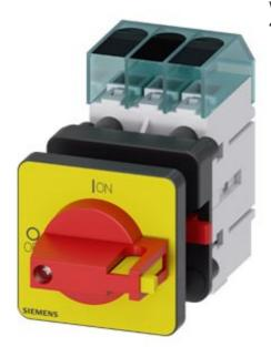
Switch disconnector 3LD3, main switch 3-polig, lu 40A operational switch at AC-23 A at 400 V 15,0 kW front mounted Base mounting with center-hole 22,5 mm knob-operated mechanism red/yellow 48 x 48 mm
