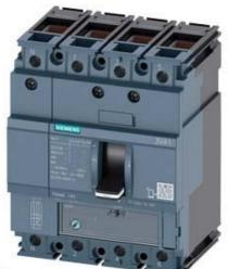
CIRCUIT BREAKER 3VA1 IEC FRAME 160 BREAKING CAPACITY CLASS S ICU=36KA @ 415 V 4-POLE, LINE PROTECTION TM220, ATFM, IN=16A OVERLOAD PROTECTION IR=11,2A ...16A SHORT CIRCUIT PROTECTION II=10 X IN NEUTRAL UNPROTECTED CABLE CONNECTION
