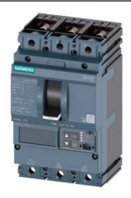
CIRCUIT BREAKER 3VA2 IEC FRAME 250 BREAKING CAPACITY CLASS H ICU=85KA @ 415 V 3POLE, LINE PROTECTION ETU560, LSIG, IN=250A OVERLOAD PROTECTION IR=100A ...250A SHORT CIRCUIT PROTECTION ISD=0,6..10X IN, II=1,5..10X IN NEUTRAL PROTECTION OPTIONAL WITH EXT. CT,UPTO 160% GROUNDFAULT, SWITCHABLE IG=0,2... 1 X IN, TG=0,050,8MS BUSBAR CONNECTION
